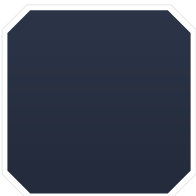
No grid lines on cell front
