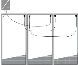
» A multiplier is required for an increased output of the PV modules. Under normal conditions, a PV module is likely to produce a higher current and / or voltage than under standardized test conditions. With such an increased power output, the requirements under Article 690 of the American safety standard NEC (National Electrical Code) must be observed.
