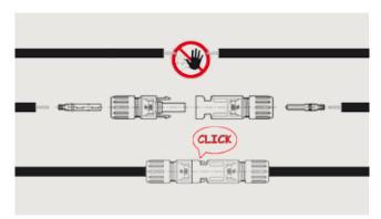
» Ensure the firm connection between the plugs. They audibly click into place when they are connected.
