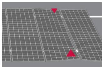
» Do not expose the modules to any mechanical tension when screwing them onto the installation system. (Torsion)
