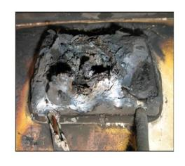
Most common failures are with opened, shorted or partially damaged Bypass-Diodes due to repeated overheating
