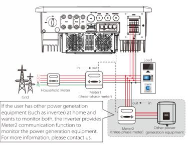
Note: If you want to connect the meter, please ground the GND terminal of the Meter1.
