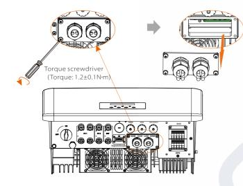
Step 3. Insert the communication cable through the communication adapter, and peel off the outer insulation layer of 15 mm.
