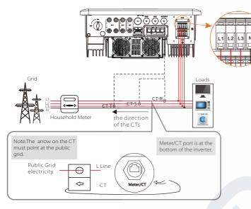
Note: CT-R must be connected to L1, CT-S connected to L2 and CT-T connected to L3 in accordance with the L1, L2 and L3 of the inverter's grid port. The household meter should be installed on the power lines.
