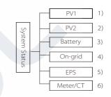
System status contains six content: PV1/PV2/Battery/On-grid (energy feed into or buy from the grid)and EPS(Off-grid) and so on. Press up and down to select, press "Enter" to confirm the selection, and press "ESC" to return to the menu.
