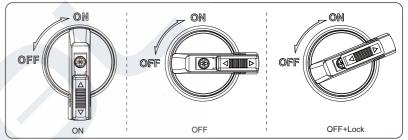
• To turn on the DC switch i) Turn on the DC switch from OFF state to ON state.
