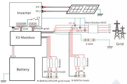
Diagram B: N line and PE line separate wiring, M series inverters; (For most countries)
