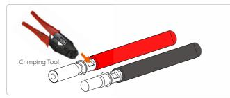
**Step 5.** The PV connectors are divided into 2 parts - the plug and the fastening head. Insert the cable through the fastening head and the opposite plug. Note that the red and black lines correspond to different of plugs. Finally, force the cable pair into the plug, will a "click" sound ,which indicates that the connection is complete.
