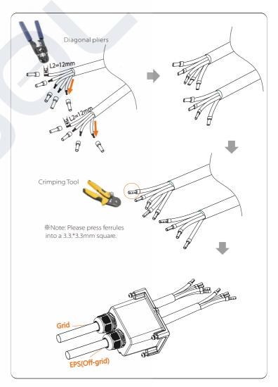
**Step 4.** Find the location of the AC interface on the inverter, insert the crimped terminals into the UW10 terminals L1, L2,L3,N, and PE according to the wire sequence, and use a flat-blade screwdriver to tighten the screws. (Torque: 1.5±0.1N·m)
