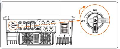
• To turn off the DC switch i) Rotate the DC switch from ON state to OFF state.
