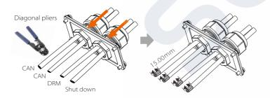
Step 4. Insert the prepared communication cables into the RJ45 terminals in sequence, and then use network cable crimping pliers to press them tightly.
