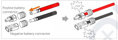
Step 6. Tighten the fastening head and into insert the corresponding positive and negative (BAT-/BAT+) ports of the inverter.
