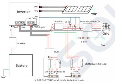
Diagram B: N line and PE line separate wiring, M series inverter; (For most countries)
