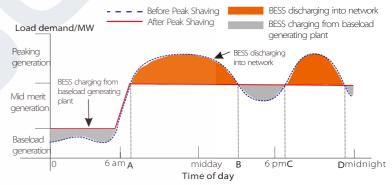
The D-A period is the battery charging period during which discharging is not allowed and the PV will charge the battery first for peak shaving. The ChargeFromGrid" setting determines whether or not to charge from the grid. When "ChargeFromGrid" is set to "Disable", the battery cannot charge from the grid; when "ChargeFromGrid" is set to "Enable" and the actual battery SOC is less than "Max\_SOC", the battery will charge from the grid at no more than "ChargePowerLimits" power.
