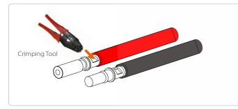
Step 5. The battery connectors are divided into 2 parts - the plug and the fastening head. Insert the cable through the fastening head and the opposite plug.
