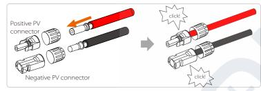
**Step 6.** Tighten the fastening head and into insert the corresponding positive and negative (PV-/PV+) ports of the inverter.
