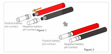
Step 4. Tighten the BAT pin needle and the wiring harness to make the connection tight without looseness.
