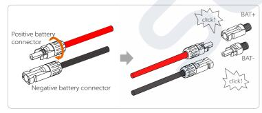
Step 7. Insert the battery power lines into the corresponding BAT port (+), (-) of the inverter.
