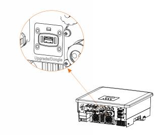
Step 2. Plug Wifi Dongle into the DONGLE port.
