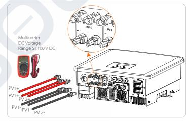
Schematic diagram of the inverter PV connected.
