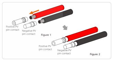
**Step 4.** Tighten the PV pin needle and the wiring harness to make the connection tight without looseness.
