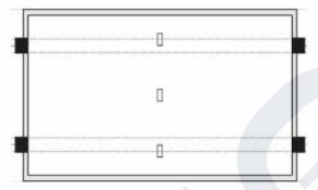
Mounted with 4 clamps along short frame. C-shaped steel parallel to the long frame. Clamp: height=30mm,width=40-50mm Maximum load: front ≤1600pa back ≤1200pa
